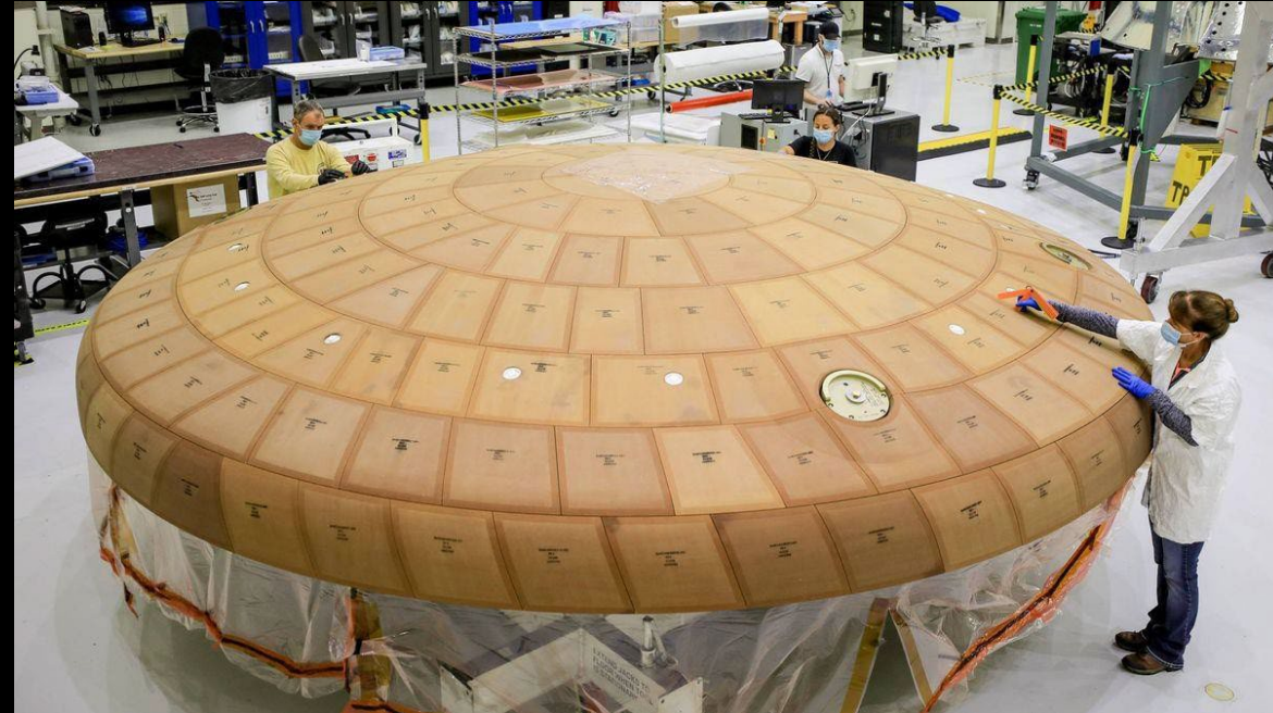
Orion's heat shield features an ablative material called Avcoat Credit: Lockheed Martin
