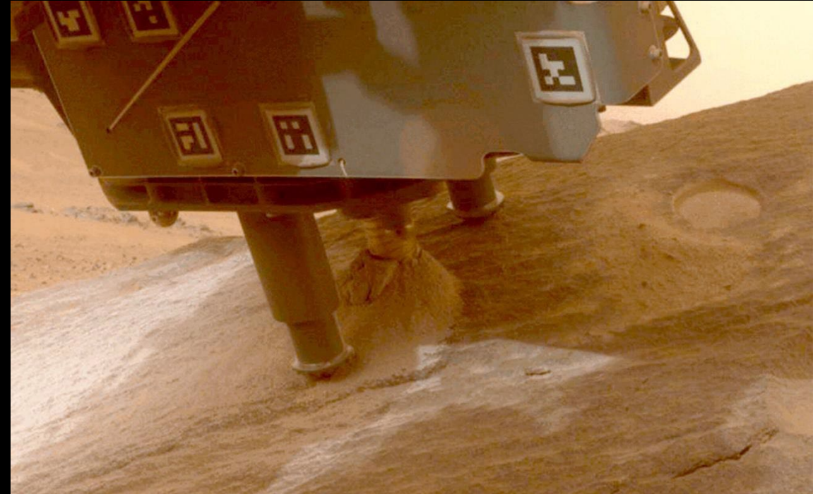
Perseverance collecting a sample from a rock called "Bunsen Peak" using a coring bit on the end of its robotic arm on March 11, 2024
